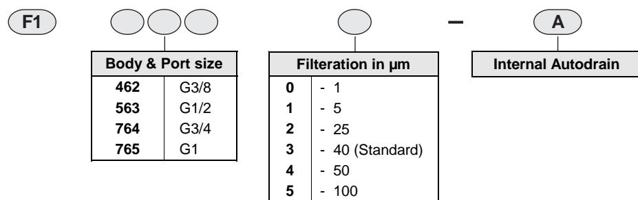
**Ordering Example** :- Filter - 3/8 size (with G 3/8 port) with a 50µm Filter with Internal Autodrain: Ordering No: F14624 - A
